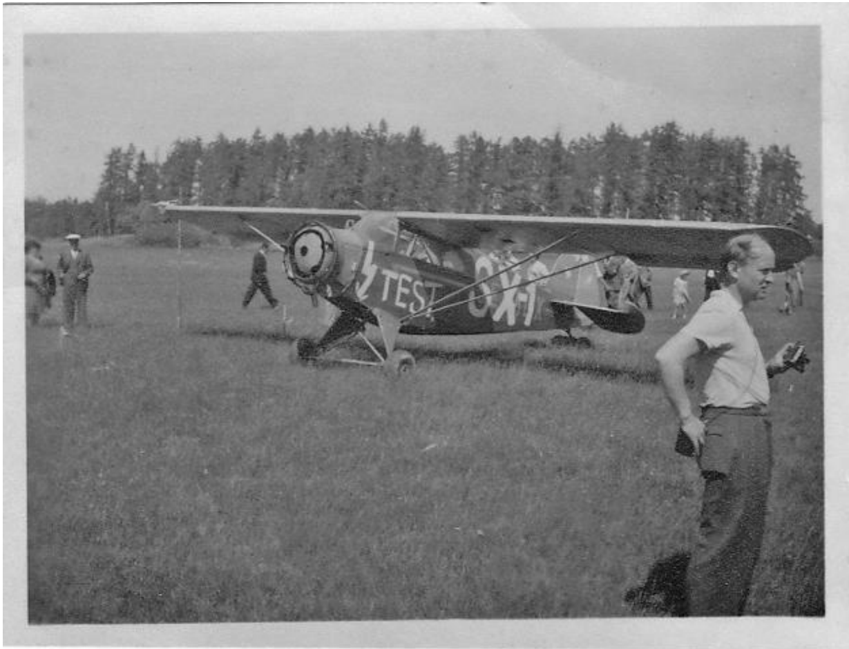
SE-AHE seen following its ‘conversion’ as a turbine jet aeroplane. Note the additional undercarriage strut. Photo: Kurt Börjesson
