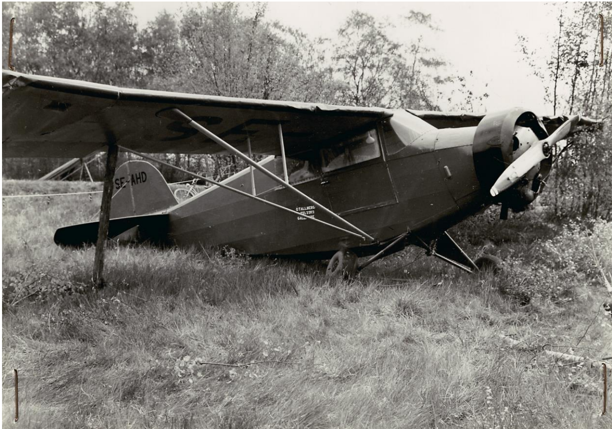
SE-AHD seen following the force landing at Laknäs. Note the temporary strut beneath the right wing. Photo: via Swedish National Archives
