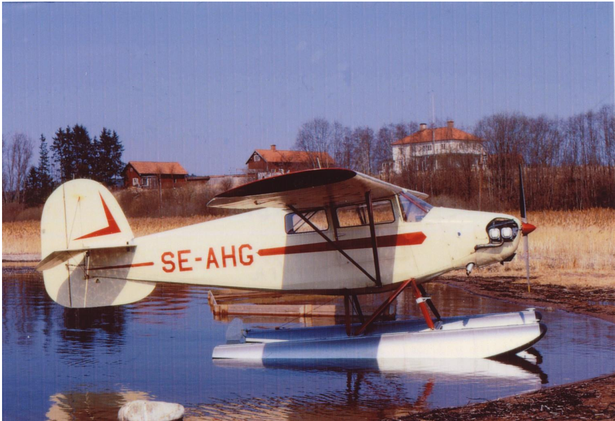
An nostalgic photo, showing SE-AHG on floats in 1974. The changed fuselage lines due to the Continental engine and lower fin are in clear evidence. This particular GV-38 is currently the sole airworthy aircraft of its kind. Photo: Leif Fredin
